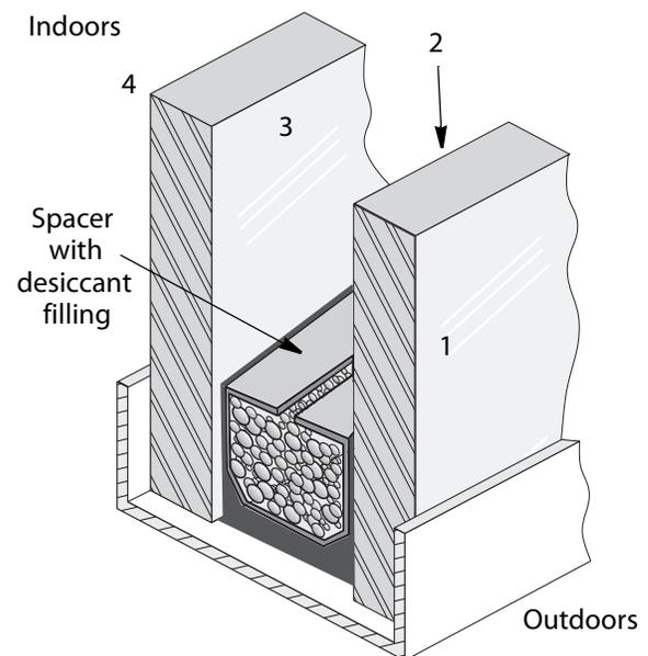
Insulated glass employs a sealed spacer between the two glass panes. A low-e coating on one pane retards emission of radiant heat from that pane. In warm climates, the coating is located on surface #2. In cold climates, the coating is located on surface #3.
