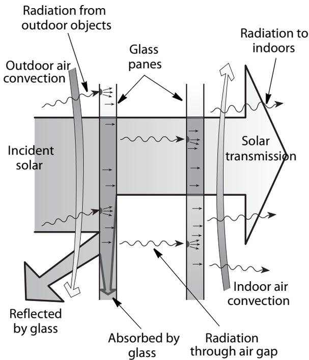
Most incident solar energy streams through the double-pane glass assembly, although some is absorbed and some is reflected. The glass absorbs most longer-wave infrared radiation from warm outdoor objects. Absorbed solar heat and heat from hot outdoor air conducts through the glass, then radiates across the air space and is absorbed by the second pane. Finally, radiation and convection carry that heat indoors.
