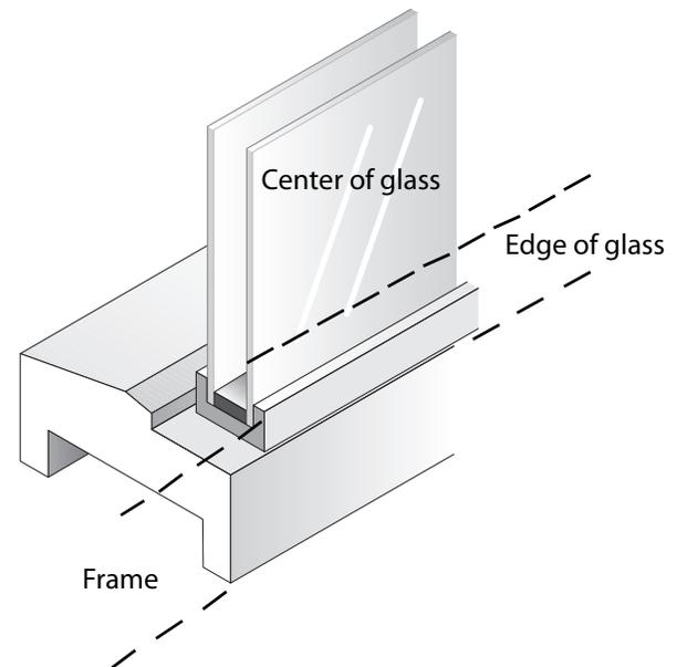
The U-factor of an insulated glass window is an area-weighted average of the window's center of glass, edge of glass, and window frame.
