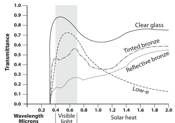
Transmittance of radiant energy varies widely with the type of glass used in a window.
