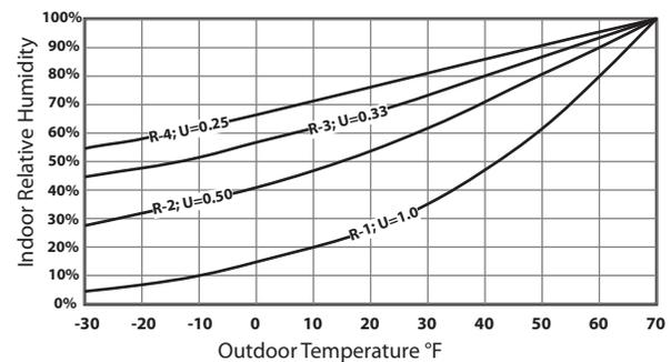
The indoor relative humidity and thermal resistance of glass determines what outdoor temperature will cause condensation.
