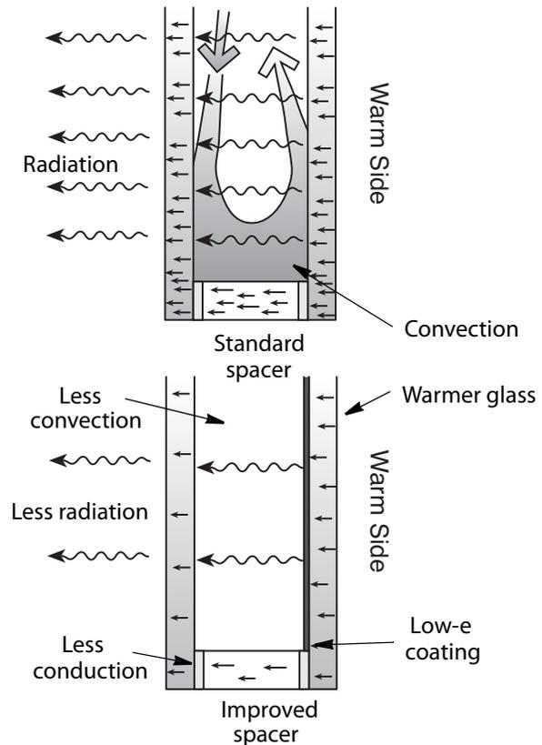
Low-e coatings reduce radiant heat flow, increasing the temperature of the warm-side glass pane. This temperature increase reduces conduction through the glass. Improved spacers reduce conduction heat flow. Heavier gases like argon reduce convection between the glass panes.
