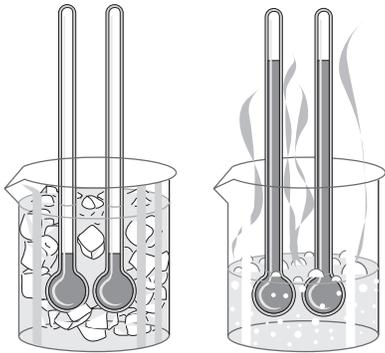
The boiling point and freezing point of water are important to calibrating thermometers because these two states are easy to recognize and duplicate. Freezing point: 32°F or 0°C; boiling point: 212°F or 100°C.
