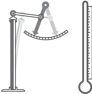
Temperature is measured by the movement of a bimetal element or by the expansion of the liquid metal mercury.
