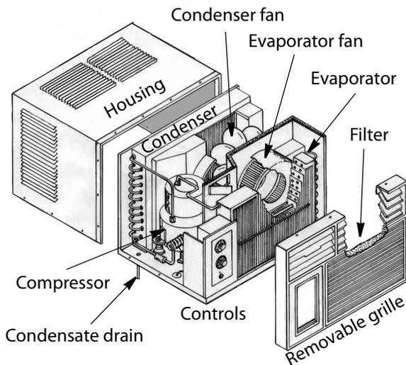
Room air conditioner performance deteriorates as it accumulates dirt. The air conditioner will eventually break down or fail to cool the room unless it is cleaned.
