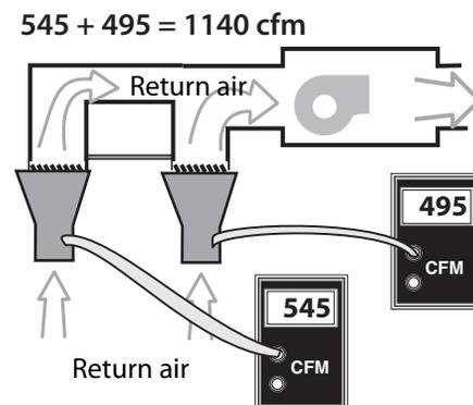
Technicians should measure airflow during a tune-up. These methods are among the most accurate for measuring airflow. Instrument calibration and the system's air leakage can affect testing accuracy.
