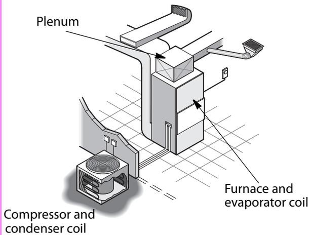
This upflow furnace has the evaporator coil in its plenum (main supply duct). The condenser and compressor are outdoors. Split system air conditioners can be a part of combustion furnaces, electric furnaces, or heat pumps.
