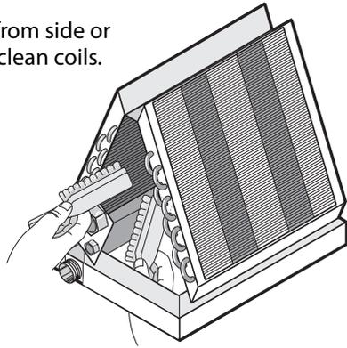
Access the a-coil from the side or underneath in up-flow systems. Clean the fins by brushing, then spraying with cleanser and rinse water, if necessary.
