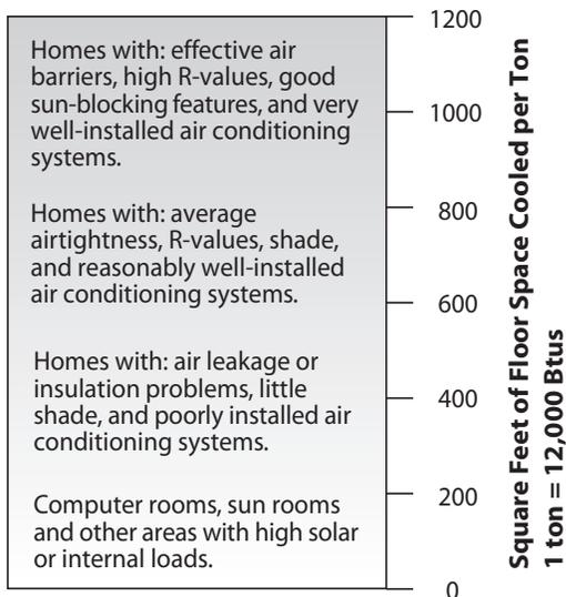
The number of square feet of floor space that can be cooled by a ton of air conditioning depends on climate, shade, insulation levels, and air leakage.
