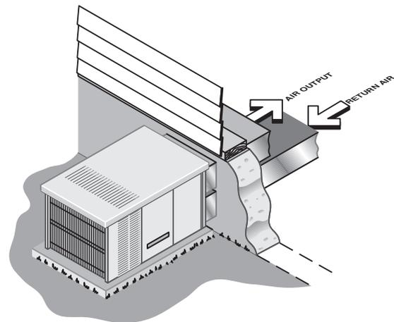
The packaged air conditioner contains an evaporator, condenser, compressor, and all the other parts in a single cabinet located outdoors. Indoor air is circulated through the evaporator and cooled, while the outdoor air absorbs the heat collected indoors.
