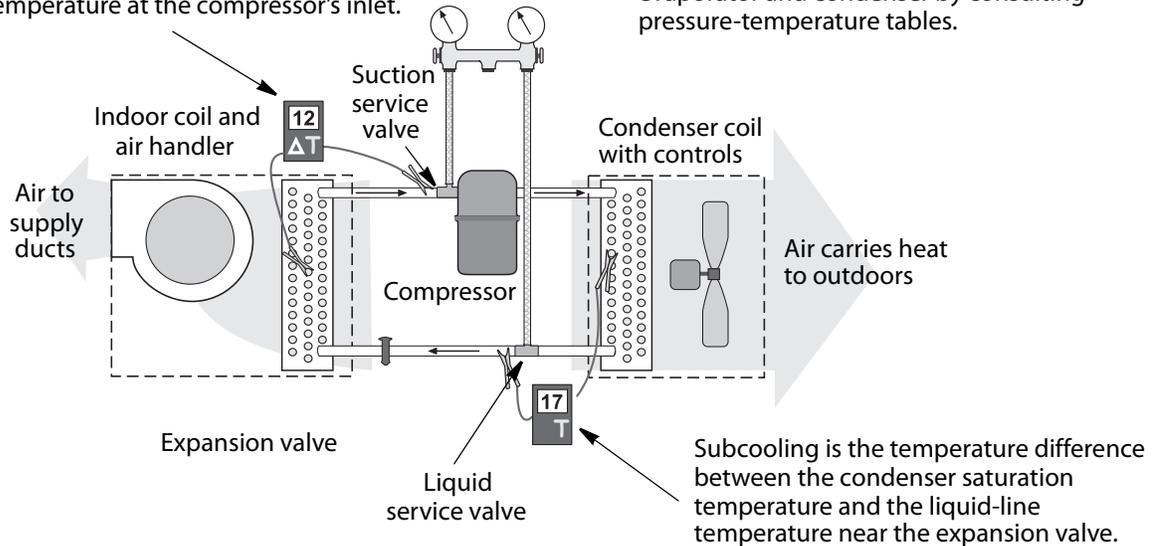
Technicians measure superheat or subcooling temperatures during summer cooling. These measurements indicate whether or not the refrigerant charge is correct.
