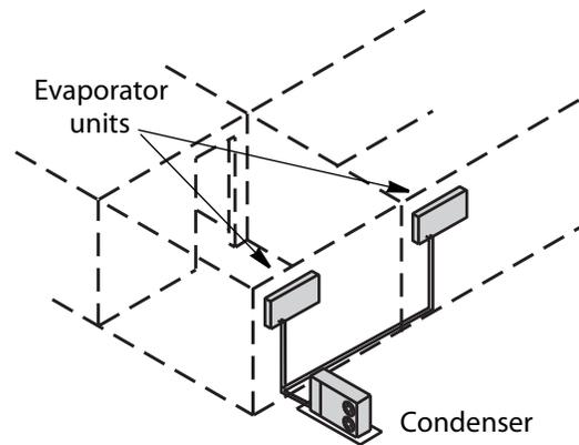
Mini-split systems employ a cooling unit—with an evaporator coil and fan—in each room. The condensing unit serves up to four indoor units.
