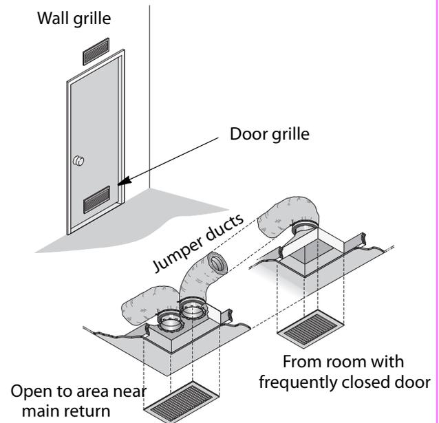
Closed interior doors create a return-air blockage in systems with only one or two returns. Grilles through doors or walls or jumper ducts can reduce house pressures, improving circulation and comfort.
