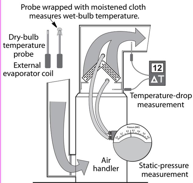
Temperature and pressure differences across the indoor coil give an indication of airflow's adequacy.
