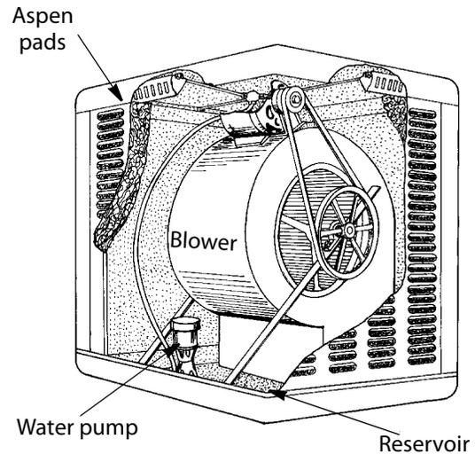
Most evaporative coolers are down-flow units mounted on the roof, but wall-mounted and ground-mounted units are easier to service.
