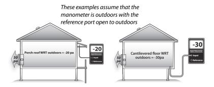
**Porch roof test:** If the porch roof were outdoors, the manometer would read near 0 pascals. We hope that the porch roof is outdoors because it is outside the insulation. We find, however, that it is partially indoors, indicating that it may harbor significant air leaks through the thermal boundary.
