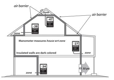
**Pressure-testing building zones:** Measuring the pressure difference across the assumed thermal boundary (*house wrt zone*) tells you whether the air barrier and insulation are aligned. If the manometer reads close to –50 pascals, the air barrier and insulation are aligned and the tested zones are well-connected to outdoors.
