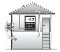
**Zone connectedness:** The attic measures closer to outdoors after the basement window is opened, indicating that the attic and basement are connected by a large bypass.
