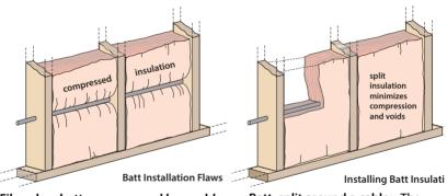
**Fiberglass batts, compressed by a cable:** This reduces the wall's R-value by creating a void between the insulation and interior wallboard.
