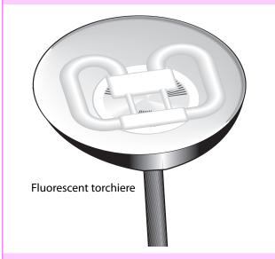
Halogen torchieres employ wattages as high as 400 watts, making them a significant heat source in summer and a fire hazard because of the high lamp temperature. Fluorescent torchieres are a logical and energy efficient replacement for these inefficient halogen incandescent lamps.
