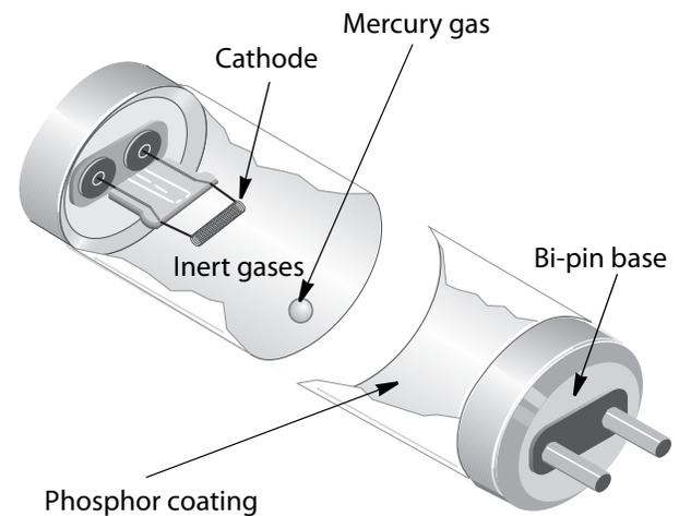
A minute amount of mercury mixed with inert gases conducts electric current, stimulating the phosphor coating on the glass tube to emit light.
