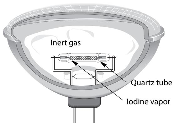
Quartz-type incandescent bulbs last longer because the quartz tube preserves the filament. The reflector design delivers more light out of the fixture toward the area needing illumination.
