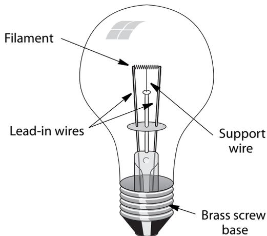
The electric circuit in the incandescent light bulb starts at the base, travels through the lead-in wires and filament, and back to the base. One lead-in wire is soldered to the base's center bottom, and the other to the brass rim.
