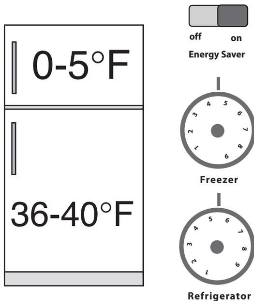
Keeping refrigerator temperatures in the range illustrated above minimizes energy use while providing adequate refrigeration. The energy-saver switch should be in the on position unless frost appears around the door, in which case, switch it to the off position.
