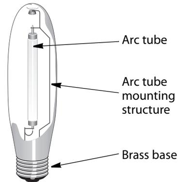
High-intensity discharge lamps, including high-pressure sodium, metal halide, and mercury vapor, have high efficacies. They have arc tubes and external ballasts.
