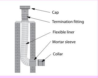
Masonry chimneys without liners or with deteriorated liners should be re-lined with a rigid or flexible chimney liner.
