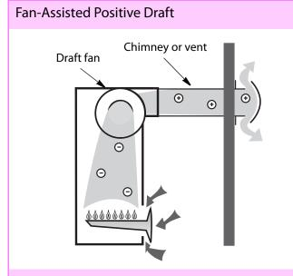
Fan-assisted positive draft is a less common venting option for modern boilers and furnaces. The chimney or vent must be airtight.
