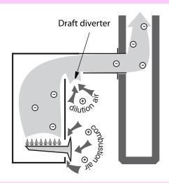
An atmospheric open-combustion heater uses only the buoyancy of the combustion gases to exhaust these gases and to pull combustion air in.
