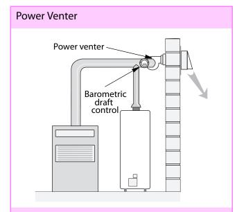
Power venters are fans located at the vent's termination. Power venters are sometimes retrofit onto atmospheric appliances to facilitate horizontal venting when a chimney is failing or absent.
