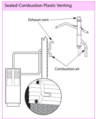
Plastic pressurized condensing vents (Category IV) can run either horizontally or vertically from the condensing appliance.
