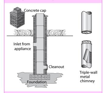
Masonry chimneys should be lined with a fireclay liner and have their own foundations.
