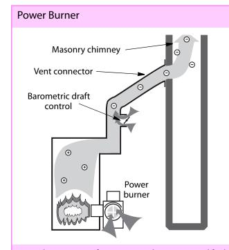
Power burners use a fan to mix combustion air and fuel thoroughly. Combustion by-products are removed by the negative draft of a masonry chimney and vent connector.
