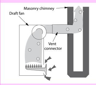
The fan-assisted appliance creates over-fire draft with a draft fan. Chimney draft is atmospheric.
