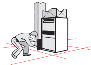
Panel filter installed in filter slot in return plenum
