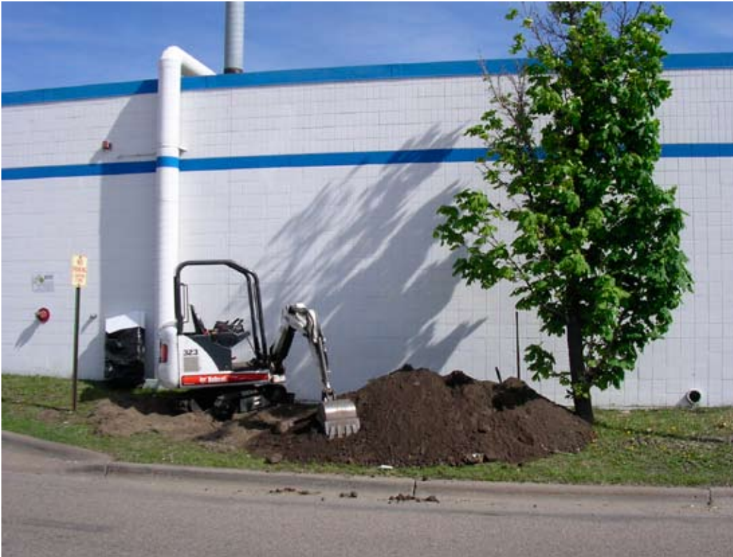
Figure 1. Excavation of insulation samples after 15 years
