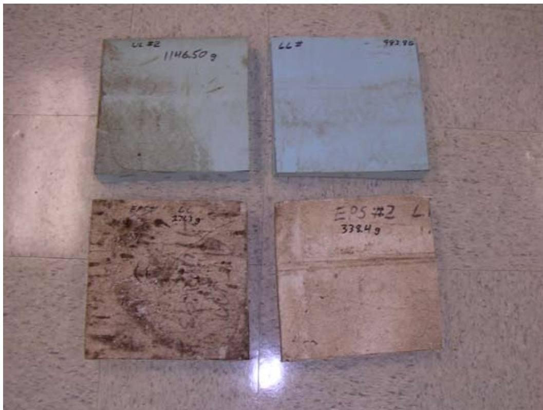
Figure 4. Samples cleaned and ready for testing
