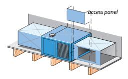
Plenums, poorly sealed to air handler: When air handlers are installed in tight spaces, plenums may be poorly fastened and sealed. Cutting a hole in the duct may be the only way to seal this important joint.
