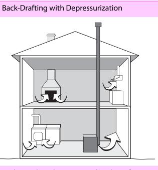
Appliances that exhaust air — such as dryers, fireplaces, and exhaust fans — create a suction that can cause the furnace chimney to back-draft indoors.
