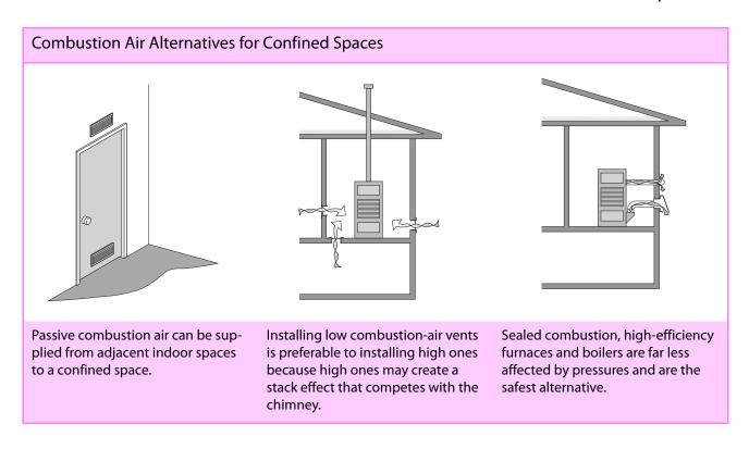
*Combustion air* — Air leakage through the building shell usually provides combustion air. Some codes and code officials require combustion air piped in from outdoors, especially for confined spaces. A confined space is a room containing less than 50 cubic feet of volume for every 1000 BTU per hour of appliance input.
