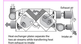
Exhaust air moves through the heat exchanger, heating its plastic or metal plates. The warm metal or plastic heats the incoming air, which moves in alternating spaces between plates, and in the opposite direction as the exhaust air.
