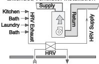
The ducted exhaust installation requires the air handler's blower to draw supply air into the home.
