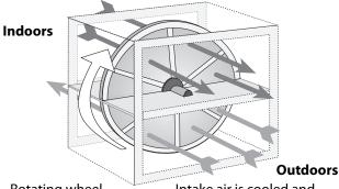
Rotating wheel transfers heat and humidity between two air streams Intake air is cooled and dehumidified in summer or heated and humidified in winter.
