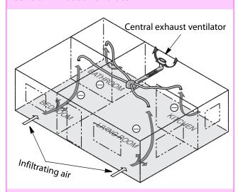
A central exhaust ventilator pulls air out of rooms and exhausts it outdoors. Make-up air infiltrates through air leaks in the building shell. The house is under a negative pressure. A central supply ventilator would be installed in a similar manner but with filtered outdoor air delivered to the home and stale air exiting through air leaks.
