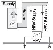
Least satisfactory of the three options, the simplified installation depends on proper duct sizing and air-handler airflow.
