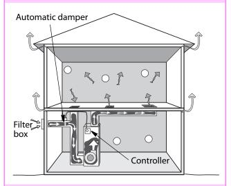
The air handler draws filtered outdoor air into the home, pressurizing it. Stale indoor air exits through air leaks in the building shell. The automatic damper opens when the air handler comes on. The controller opens and closes the damper and cycles the air handler as needed to ventilate the home.
