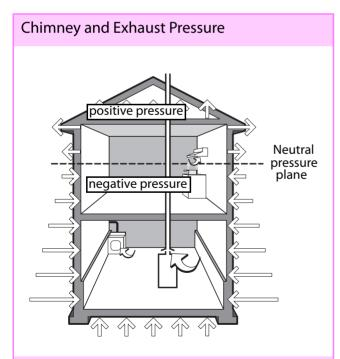
The chimney, clothes dryer, and kitchen exhaust fan exhaust air from the home, putting most of the home's volume under negative pressure. The wind creates a vacuum at wall and roof surfaces parallel to its flow. The leeward side, facing away from the wind, is usually either neutral or depressurized.
