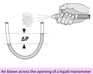
creates a vacuum in the tube and a measurable difference in the height of the water level. This  $\Delta P$  depends on the air velocity and is used to calculate airflow in CFM.
