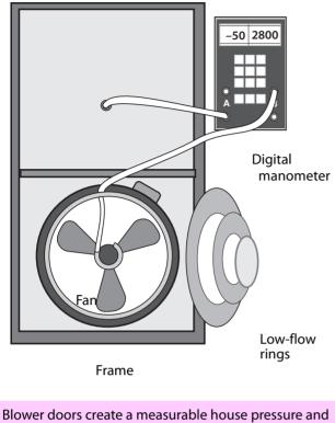
Blower doors create a measurable house pressure and airflow in order to evaluate a building's air leakage.
