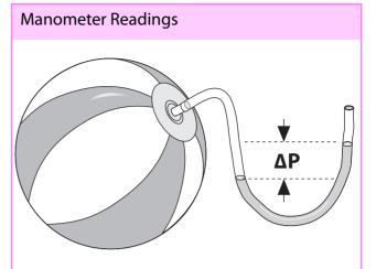
The pressure inside an inflated beach ball is greater than the pressure of the atmosphere. This pressure difference ( $\Delta P$ ) can be measured with a manometer showing how many inches the water level differs in its height. This is the origin of the measurement: inches of water column (IWC).
