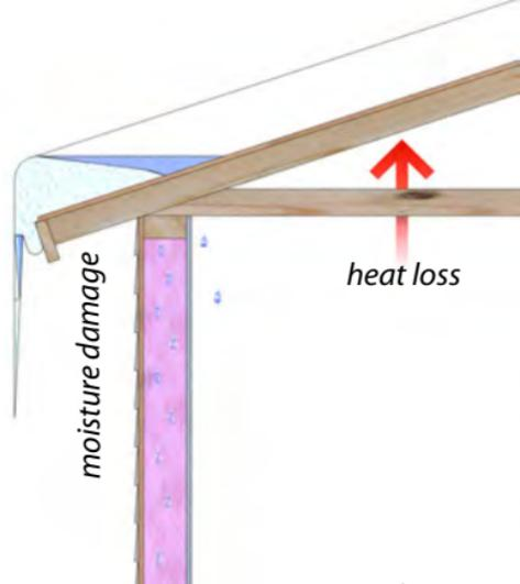
**Ice damming:** When a roof is unventilated, the home's heat loss warms the roof deck melting snow. The water re-freezes at the eaves and causes moisture damage.
