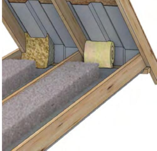
**Insulation at the eaves:** Stuff fibrous insulation into the eave area to maximize R-value. Use mechanical fasteners to attach the baffles to the framing.
