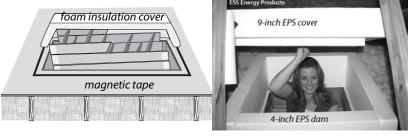
**Manufactured pull-down-stair covers:** Manufacturers provide insulated stair covers for use with walkable attic floors or with dams to be surrounded by fibrous insulation.
