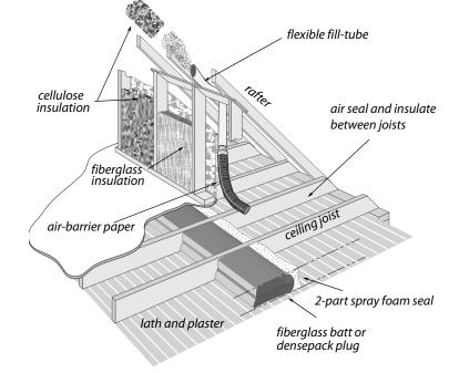
**Finished attic best practices:** Air sealing and insulation combine to dramatically reduce heat transmission and air leakage in homes with finished attics.
