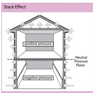
The stack effect is caused by the relative buoyancy of warmer air. Warmer air's upward force exerts an outward pressure. Airflow, through holes in the home's top, creates suction at lower levels, pulling air in. Arrows indicate the direction and intensity of air pressure.
