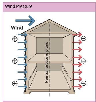
Wind creates a positive pressure on the windward side of the home and negative pressures on leeward side with reference to the home's interior. Wind pressures push and pull air through holes in the building shell.
