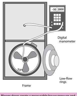
Blower doors create a measurable house pressure and airflow in order to evaluate a building's air leakage.
