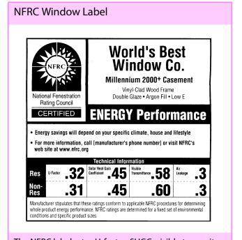
The NFRC label rates U-factor, SHGC, visible transmittance, and air leakage. Manufacturers associated with NFRC must submit their products for testing.
