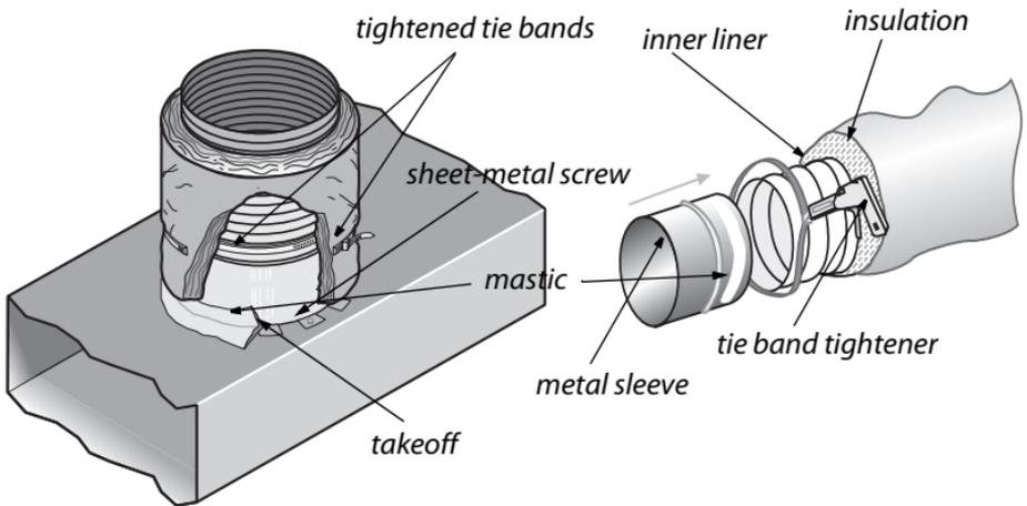
**Flexduct joints:** Flexduct itself is usually fairly airtight, but joints, sealed improperly with tape, can be very leaky. Use methods shown here to make flexduct joints airtight.
