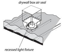
Air seal and shield for non-IC can: This drywall box is an insulation shield and air seal, but allows the fixture some air circulation for cooling.
