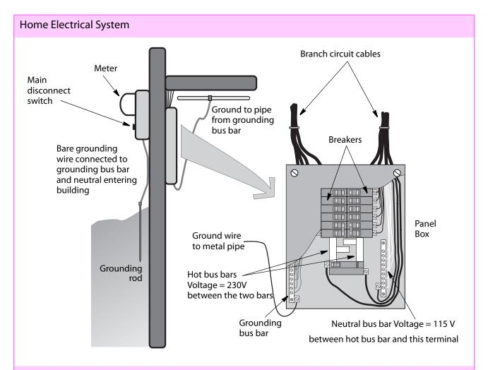
The major parts of a home electrical system are the service panel and the distribution panel box. The service panel contains the meter and main switch. The distribution panel box contains the breakers or fuses, and the power, neutral, and grounding, bus bars.
