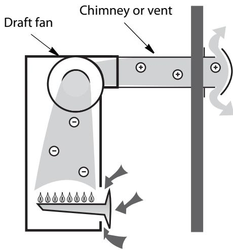
Fan-assisted positive draft is a less common venting option for modern boilers and furnaces. The chimney or vent must be airtight.
