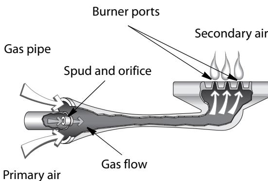
The most common type of burner is the atmospheric-gas burner for burning natural gas or propane.
