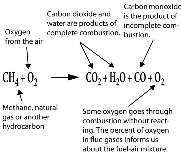
Combustion is a heat-yielding chemical reaction starting with a hydrocarbon and oxygen and producing  $\text{CO}_2$  and water as its ideal products.
