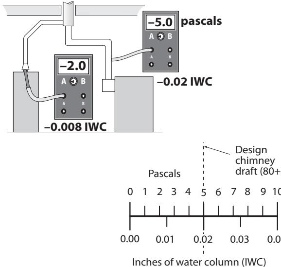
Measuring chimney draft gives important information about the combustion process.
