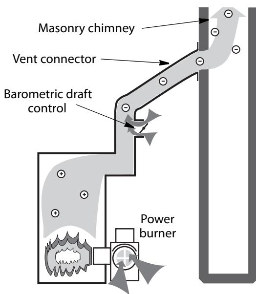
Power burners use a fan to mix combustion air and fuel thoroughly. Combustion by-products are removed by the negative draft of a masonry chimney and vent connector.
