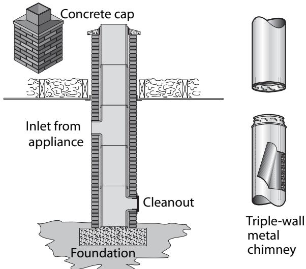
Masonry chimneys should be lined with a fireclay liner and have their own foundations.
