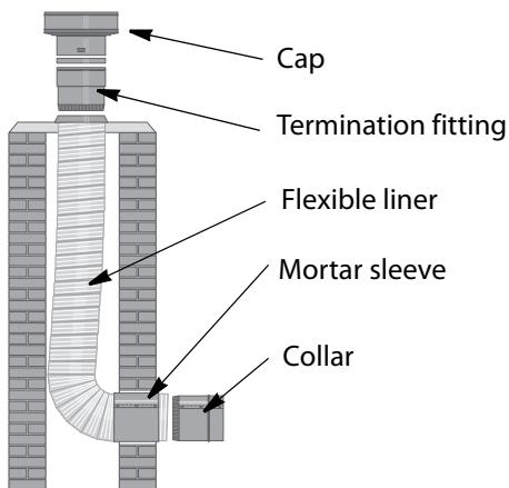
Masonry chimneys without liners or with deteriorated liners should be re-lined with a rigid or flexible chimney liner.
