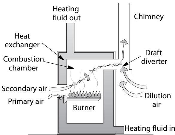
Atmospheric-draft heaters use only the buoyancy of the combustion gases and the flame's heat to exhaust combustion by-products into the chimney and pull combustion air into the burner.
