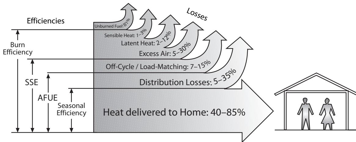
Much of the heat contained in the fuel never reaches the living space as useful heat. Fuel-burning efficiency counts losses from incomplete combustion. Steady-state efficiency (SSE) counts chimney losses. Annual fuel utilization efficiency (AFUE) counts cycling and jacket losses. Seasonal efficiency counts distribution losses in addition to the others and would be the lowest efficiency (40% to 85%).
