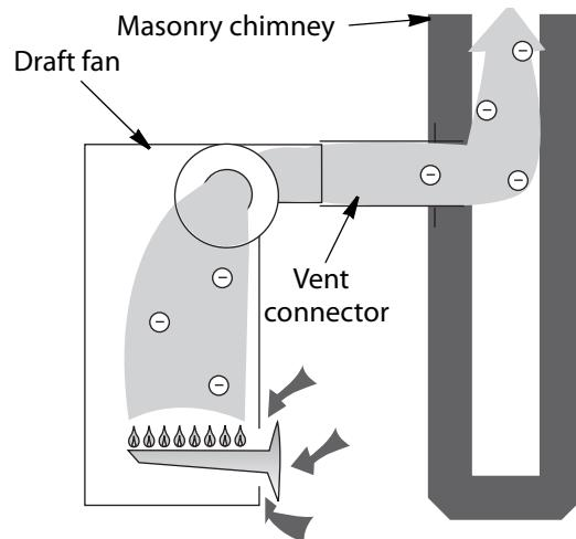
The fan-assisted appliance creates over-fire draft with a draft fan. Chimney draft is atmospheric.
