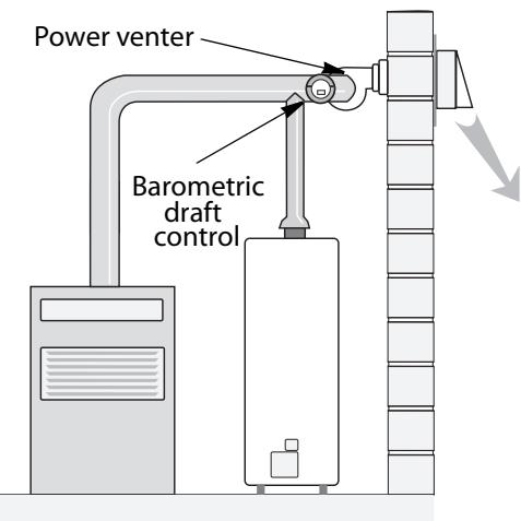
Power venters are fans located at the vent's termination. Power venters are sometimes retrofit onto atmospheric appliances to facilitate horizontal venting when a chimney is failing or absent.
