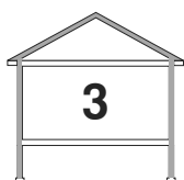
Thermal boundary encloses entire building shell
