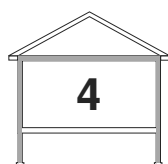
Thermal boundary encloses conditioned space and crawl space
